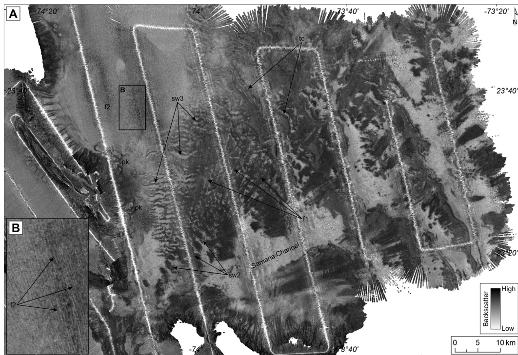
Fig. 12. Enlargement of the backscatter image of the San Salvador turbidite system. Low reflectivity corresponds to light tones; high reflectivity corresponds to dark tones. f1, f2: furrows; pk: pockmarks; sw2 and sw3: sediment waves; tc: tension cracks. B: Enlargement of the map showing furrows f2. See Fig. 1B for location.
